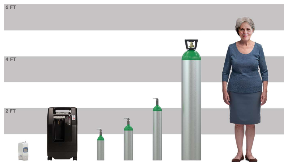
Figure 1 From left to right. Portable oxygen concentrator (4 lb, ~2 L/min), stationary concentrator (35 lb, 10 L/min), M-6 cylinder (2.2 lb, 164 L capacity), M-15 cylinder (5.3 lb, 425 L capacity), M-24 cylinder (7.9 lb, 680 L capacity), M-250 cylinder (114 lb, 7080 L capacity), average-sized woman requiring LTOT. (The individual depicted here is AI generated; it does not depict a person living or deceased.) AI, artificial intelligence; LTOT, long-term oxygen therapy.
